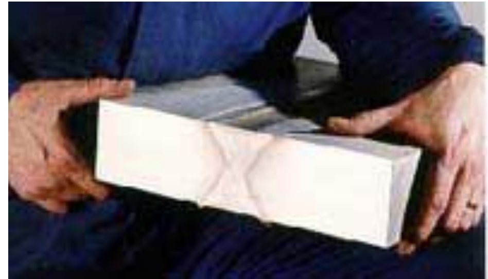
Double sided friction stir weld in 75 mm thick aluminium plates produced at TWI
